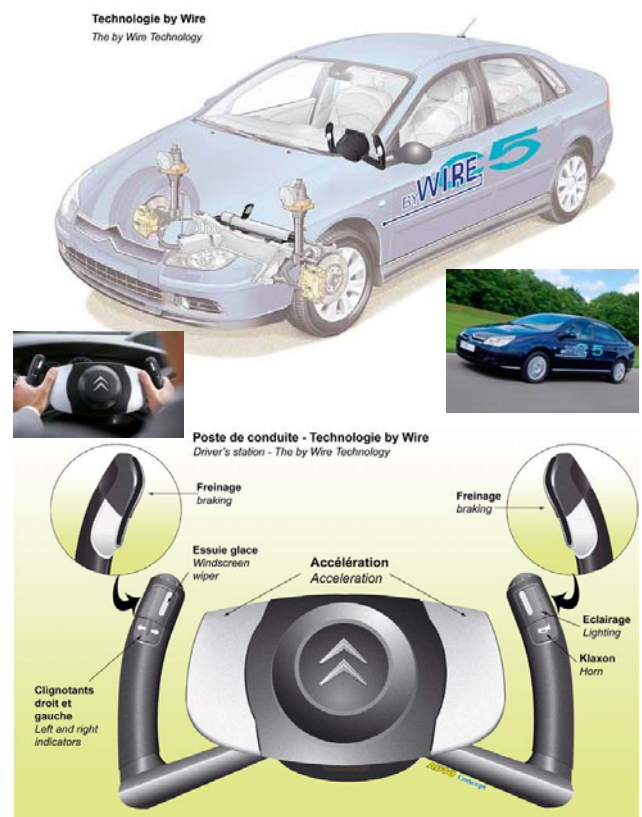
Fig.: Citroën C5 Steer-by-Wire System.
